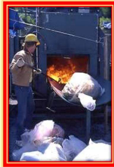
Worker feeds incinerator bagged oily debris. Dayville Incineration Site, Valdez (R6348-SR612- AS17959-0683)
